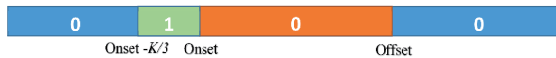
Figure 7. Frame label annotation diagram. The blue rectangle represents an entire video, and the orange part means the ME sequence. Frames in the range [\text{onset} - K/3, \text{onset}] are classified in label 1 and the rest frames are labeled in 0.
