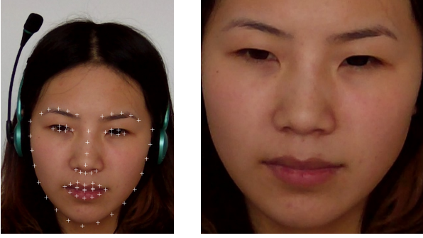
Fig. 1. Left: detection of 66 feature points in a facial region using the DRMF method. Right: the normalized facial area.
